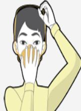
Secure ties, loops or straps and mould metal piece over nose.
